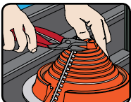
1. Using tin snips, cut the cone to fit pipe.
