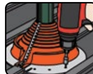
5. Fasten Retrofit to roof
